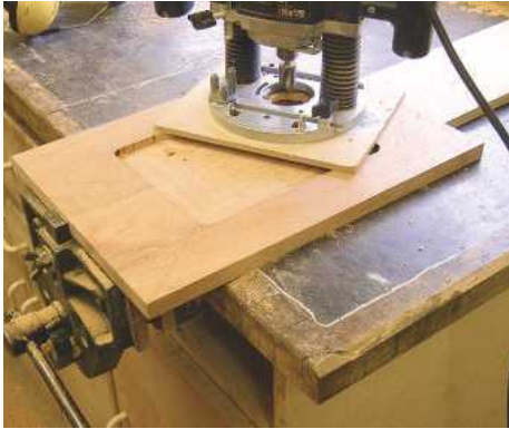
▲ Pic.13 The marquetry panel sits in a rebate routed in the top panel; the large sub-base on the router prevents it tipping
